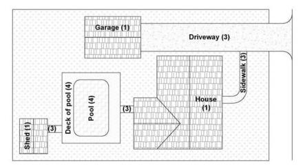
This diagram is to assist in identifying the various items considered impervious.
